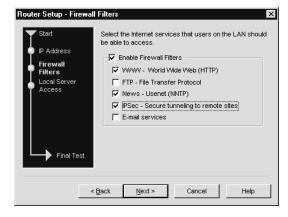
Figure 17. Set up a firewall and filters.
